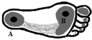
Fig. 4. Force sensors position and force applied on the foot
